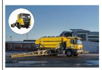
The ASP is a high quality spraying machine that ensures a fast, exact and precise application of de-icing agents. The ASP can be used for both preventive and curative de-icing on runways, taxiways and aprons, and offers a working width of up to 40 m.
