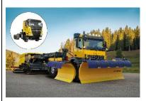
The towed TJS jet sweeper is hard to beat in terms of performance and flexibility. A clearing width of up to eight metres, excellent manoeuvrability and high working speed enable very fast and highly efficient snow clearance at airports.
